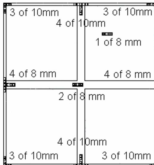
Figure No. 4: A plan of the improved design for a masonry house
